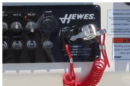
Engine Stop Switch
