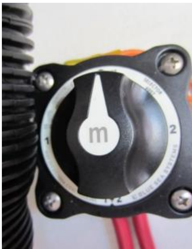
Battery Switch, Shown in the “Off” Position
