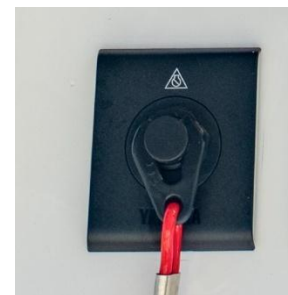
Engine Stop Switch
