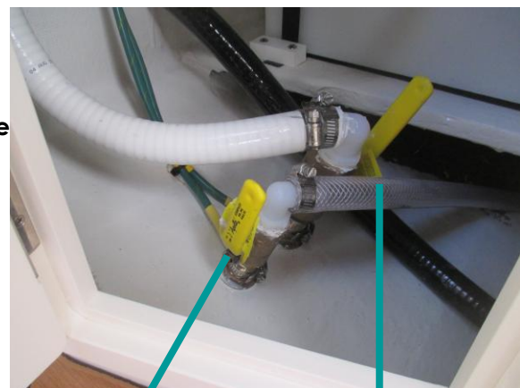
Intake Valve (open)
