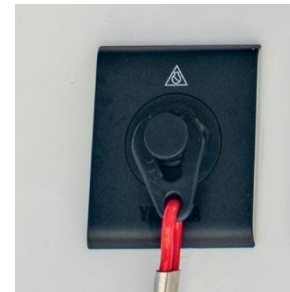
Engine Stop Switch
