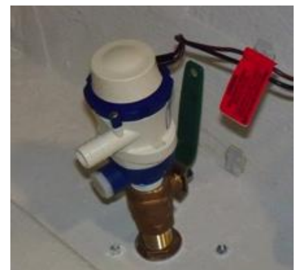
Livewell Pump Assembly in the “OPEN” Position
