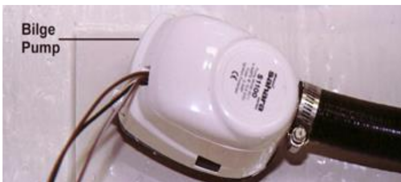
Bilge Pump is Mounted to ABS Plastic
