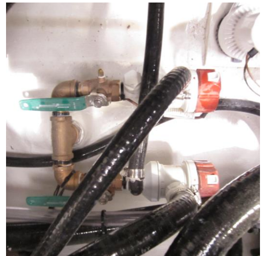
Livewell Pump Assembly in the "OPEN" Position
